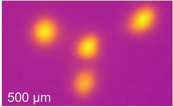
An X-ray image of the electron beam in TRIB-mode where two orbits co-exist: the regular orbit and the second one winding around it closing only after three revolutions. Credit: F. Armborst/K. Holldack/HZB
