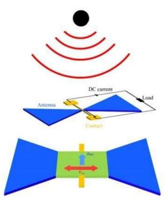
This schematic figure, from the researchers' paper, shows a green square that represents graphene on top of a square of another material. The red lines represent terahertz waves. The blue triangles represent antenna that surround the square to capture the terahertz waves and focus the waves to the square. Credit: Massachusetts Institute of Technology
