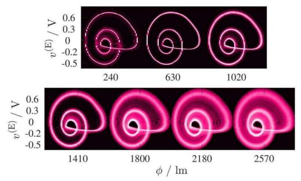
As a function of the light intensity, the dynamics of each sensor node could change from periodic (weak illumination) to markedly chaotic (strong illumination). Reconstruction of the temporal trajectory of the signal (known as attractors) revealed a characteristic snail-like shape, which was similar among the physically-realized boards, and boards thus allowed synchronization to arise between them. Credit: Minati L
