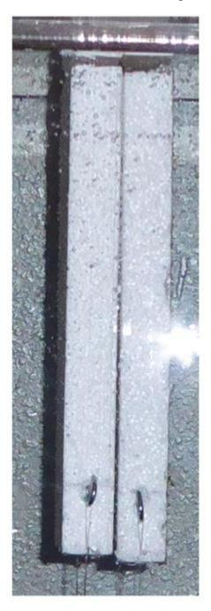
Fig. 1 Two Styroform boards in water. They separate more at the bottom than at top
