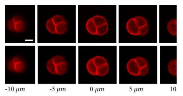
The researcher compared two-photon microscopy images of a pollen grain using traditional raster scanning (a) and their new compressive imaging approach (b). The raster-scanning imaging time was 2.2 seconds while the compressive imaging time required only 0.55 seconds. Credit: Shih-Chi Chen from The Chinese University of Hong Kong
