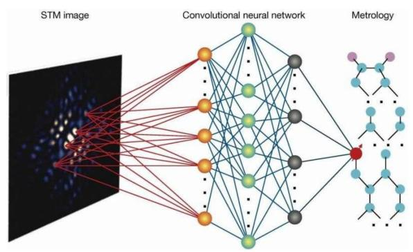
Computed scanning tunneling microscope (STM) images of phosphorus atoms qubits in silicon used to train a convolutional neural network (CNN), capable of autonomous and high-throughput qubit characterization with an exact atom precision in both, their spatial locations and atom count. Credit: M.Usman/ University of Melbourne
