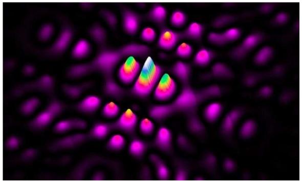
A map of electron wave function patterns, where the symmetry, brightness and size of features is directly related to the position of a phosphorus atom in silicon lattice. Credit: M.Usman/University of Melbourne
