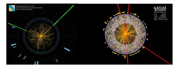
The image of the left shows two gamma rays emerging from the CERN LHC CMS detector, while the one on the right shows the tracks of four muons in the CERN LHC ATLAS detector. This time it was not the experimentalists but the *theorists* (Englert and Higgs<sup>3</sup>) who got the Nobel Prize for it: their research goes
