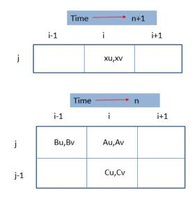
$$xu = Au - \frac{\Delta t}{\Delta x} Au(Au - Bu) - \frac{\Delta t}{\Delta y} Av(Au - Bu)$$
