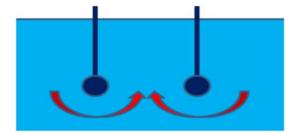
After a short time, both pendulums will oscillate in the same direction and with the same frequency!!!
