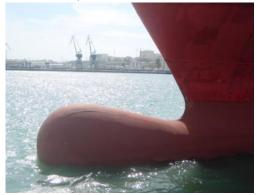
Nowadays, big ships and also small ones, have the lower part that is submerged, a bulb in the front. The function of this bulb is to create a series of waves or turbulence, which when joined with the waves generated by the boat itself, are annulled or at least almost eliminated. In this way, they greatly reduce the drag of the boat. This front bulb, is placed in front of the boat, as a kind of advance, as opening the way, as smoothing the way of the boat that comes behind.
