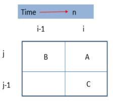
$$X = A - c \frac{\Delta t}{\Delta x} (A - B) - \frac{\Delta t}{\Delta x} (A - C)$$
