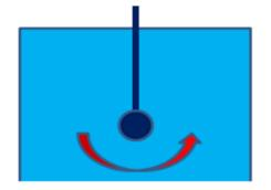
It will be able to see that the pendulum will stop oscillating almost immediately. This is due to the opposition of the water molecules which act on it. In fact, the more density/viscosity the fluid has (less compressibility), the less time the initial oscillation will take to stop.
