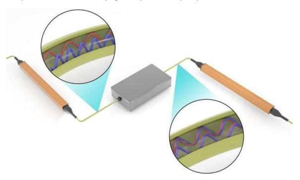
The researchers' innovative experimental setup involved operating on photons contained within a single fiber-optic cable. This provided stability and control for operations producing entangled photons, shown separated at top and intertwined ... <a href="mailto:more">more</a>"We were able to extract more information about the quantum state of our experimental system using Bayesian inference than if we had used more common statistical methods," Williams said.
