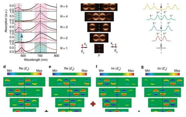
Plasmonic encoding in gold nanodisk chains. a Calculated absorption spectra of gold nanodisk chains consisting of different numbers of nanodisks illuminated by the s-polarized in-plane plan wave coming from right side (dashed line) or both ...<u>more</u>
