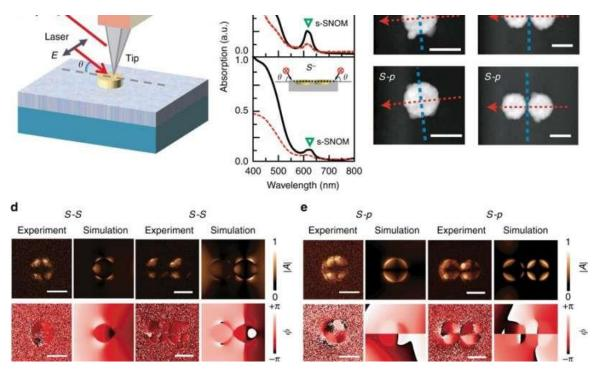
Demonstration of electrical-field distribution rule for the 200 nm gold nanodisk monomer and dimer by s-SNOM. a Schematic of the s-SNOM measurement for s–s and s–p excitation–collection configurations. The wavelength of the excitation laser ...<u>more</u>
