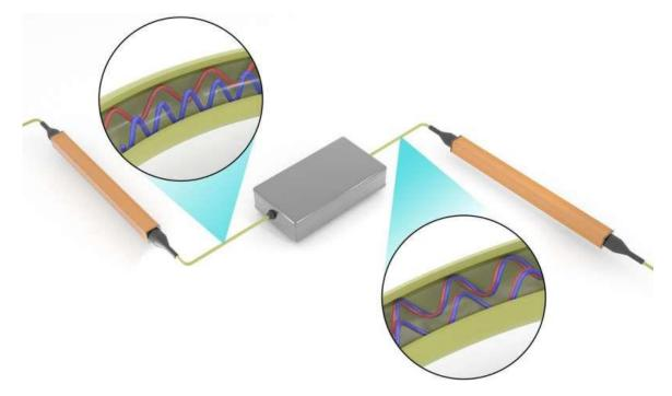
The researchers' innovative experimental setup involved operating on photons contained within a single fiber-optic cable. This provided stability and control for operations producing entangled photons, shown separated at top and intertwined ...more "We were able to extract more
