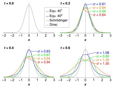
**Figure 5** | Visualizations of the time-dependent diffusion trend of a Gaussian wave packet (norm) as predicted using four methods (for Equ. 40<sup>1</sup>, the initial condition is  $\mathcal{M}_0(x,0) = 10^{-13} e^{-2x^2}$ ; for Equ. 40<sup>2</sup>, the initial condition is  $\mathcal{M}_0(x,0) = e^{-2x^2}$ ) in natural units at various moments in time ( $t = 0.0, 0.2, 0.4, \text{ and } 0.6 \text{ eV}^{-1}$ ).
