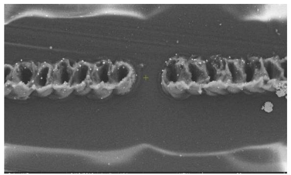
A scanning electron microscope image shows two traces of laser-induced graphene on a polyimide film. A laser mounted to the microscope was used to burn the patterns into the film. The technique shows promise for the development of flexible electronics. Credit: Tour Group/Rice University
