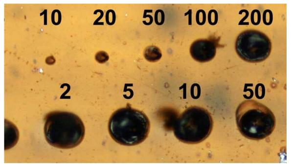
Scientists at Rice University and Oak Ridge National Laboratory used a small laser mounted to a scanning electron microscope to form dots and traces of conductive graphene on a polymer. The technique creates laser-induced graphene with features more than 60% smaller than the macro version and almost 10 times smaller than typically achieved with an infrared laser. Credit: Tour Group/Rice University
