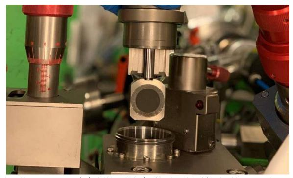
Evan Groopman, a research physicist, inserts Nuclear Signatures Inter-laboratory Measurement Evaluation Program (NUSIMEP-9) uranium particles on a carbon planchette into the NAUTILUS to analyze the uranium isotopic composition in the Accelerator Mass Spectrometry Laboratory at the U.S. Naval Research Laboratory in Washington, D.C., Sept. 5. Credit: U.S. Navy photo by Nicholas E. M. Pasquini
