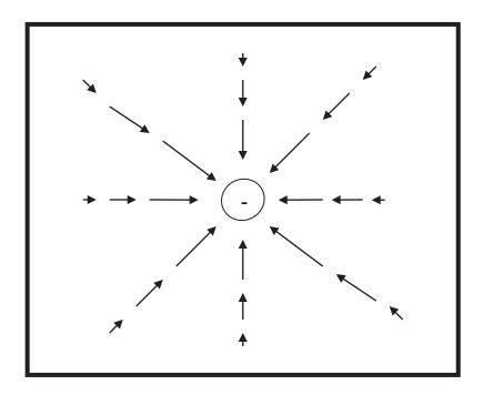
Fig 2 | Electric field's intensities in Space generated by a negative Electric Charge
