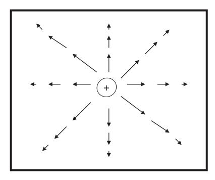
Fig 1 | Electric field's intensities in Space generated by a positive Electric Charge
