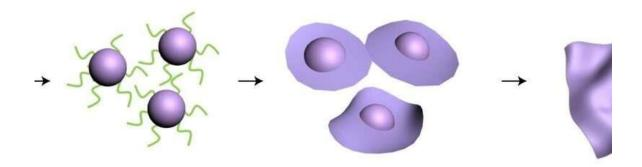
Schematic illustrating the growth of 3-D nanoparticles from a solution, and the 3-D nanoparticles transformation into 2-D nanosheets. Credit: Haimei Zheng/Berkeley Lab
