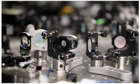
A network of optical devices -- mirrors, beamsplitters, and optical fibres -- weave laser light into an optical quantum processor. Credit: CQC2T
