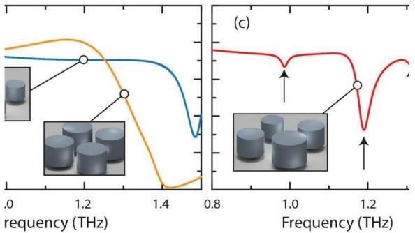
When the frequency responses of dielectric metamaterial setups consisting of four small cylinders (blue) and four large cylinders (orange) are combined into a setup consisting of three small cylinders and one large cylinder (red), the resulting response looks nothing like a straightforward combination of the original two. Credit: Willie Padilla, Duke University
