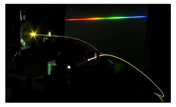
An ultrashort pulse is sent into an optical fibre and produces new frequency components via intense light-matter interactions. The progressive spectral broadening of the initial light pulse occurring during propagation, ultimately leads to ...<u>more</u>
