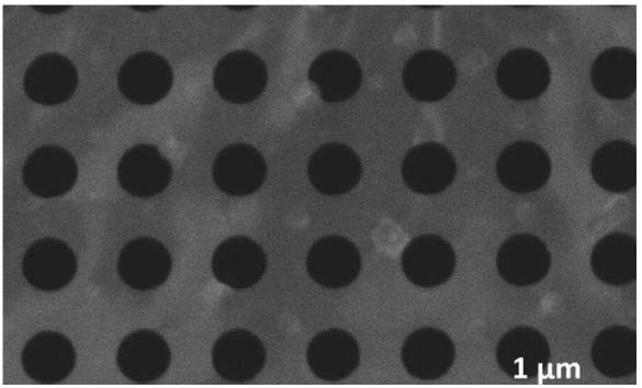
SEM image of the waveguide structure: a suspended tungsten disulfide monoloayer patterned with nanosized holes. Credit: Cubukcu lab
