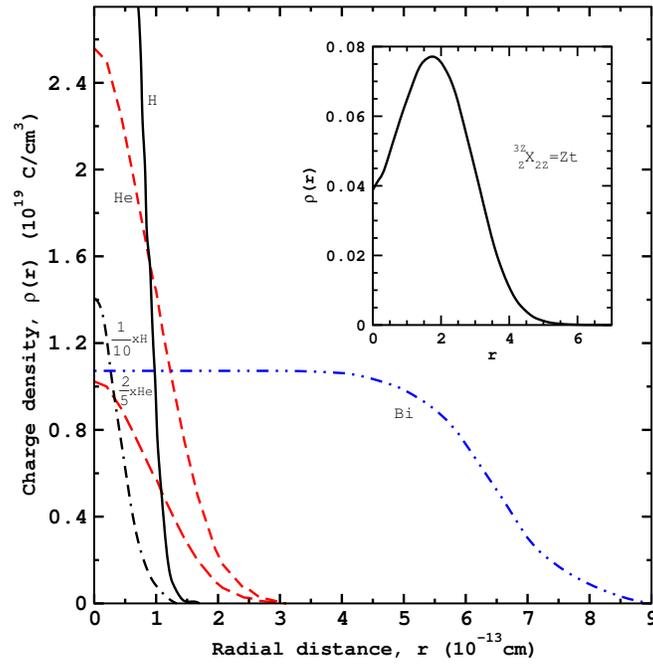
Figure 1: Schematic density distribution of nuclei as determined by electron scattering. Inset (t for triton) shows the same with a marked "hole" at the centre as that of the core of the halo nucleus, and what is called a tennis-ball (bubble) like structure. Note the basic difference between the two
