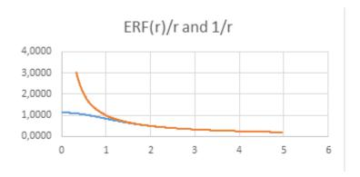
Due to the convolution, and the coherence of the location density distribution, the blue curve does not show any sign of the singularity that is contained in the red curve.
