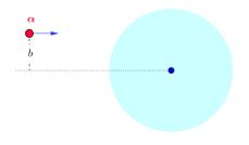
Figure 2: Rutherford's experiment - Impact parameter b
