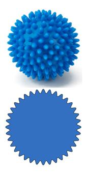
Figure 4: Particle with wavy surface and relative diametral section
