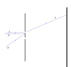
Figure 6: Possible traces of electrons in a fog chamber. Electron A passed by the upper slit. Electron B bounces from the edges. Figure not in scale.
