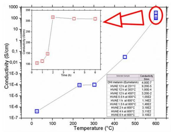
Conductivity of vacuum annealed eumelanin thin films vs. the annealing temperature and (inset) vs. the annealing time at 600°C temperature. All the measurements were performed in air at room temperature. Errors of each point are indicated inside the plots symbols. Copyright © 2019 Migliaccio, Manini, Altamura, Giannini, Tassini, Maglione, Minarini and Pezzella. Front. Chem., 26 March 2019 https://doi.org/10.3389/fchem.2019.00162
