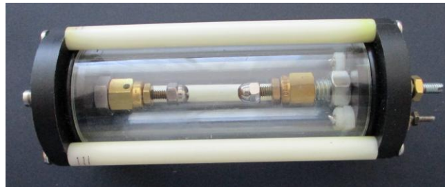
Fig 7. Vacuum cell with two glow discharge electrodes
