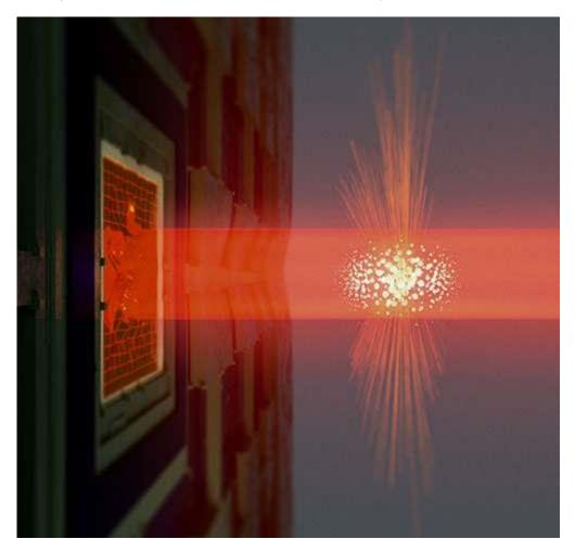
If laser light used to measure motion of a vibrating membrane (left) is first transmitted through an atom cloud (center) the measurement sensitivity can be better than standard quantum limits envisioned by Bohr and Heisenberg. Credit: Bastian Leonhardt Strube and Mads Vadsholt
