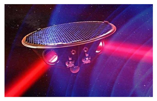
The proposed LISA mission will detect gravitational waves in space using a trio of satellites, separated by millions of kilometers. Lasers will be employed to measure the minute changes in their relative distance induced by impinging ...more
