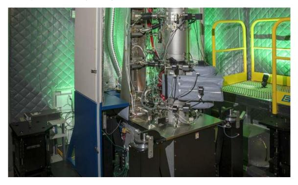
Oak Ridge National Laboratory scientists used a monochromated, aberration-corrected scanning transmission electron microscope, or MAC-STEM, technique that detects the subtle changes in the weight of proteins at the nanoscale--while keeping ...<u>more</u>"Now, we can track isotopic labels directly with the electron microscope, meaning we can do it with a spatial resolution comparable to the actual size of the proteins," Hachtel added.
