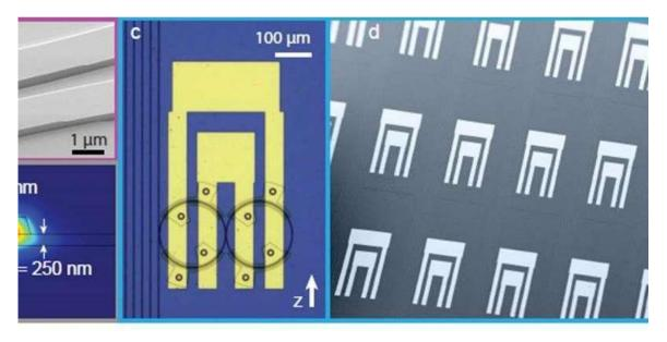
Device and experimental setup detail. a) Scanning electron microscope (SEM) image of the gap between the coupled microring resonators. b) Cross-section of the optical mode profile in the ring resonator. c) Microring image of the full device ...<u>more</u>
