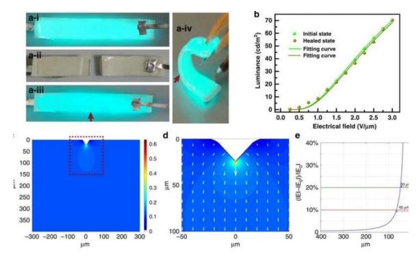
Characterizing the initial healing response: light-emitting performance of the self-healed EL device after cutting-healing process. a Demonstration of cutting–healing process of the healable EL device. a-i–a-iii exhibits the initial working ...more
