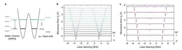
Microwave dressed photonic waveguides. a) When the applied microwave frequency is tuned to match the mode separation, dissipative coupling leads the two photonic levels to split into four levels. This effect is analogous to Autler–Townes ...<u>more</u>
