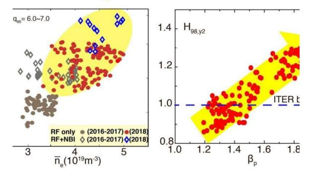
The extension of EAST operation scenario in 2018, with the comparion of its energy confinement enhanced factor to the ITER baseline scenario. Credit: EAST Team
