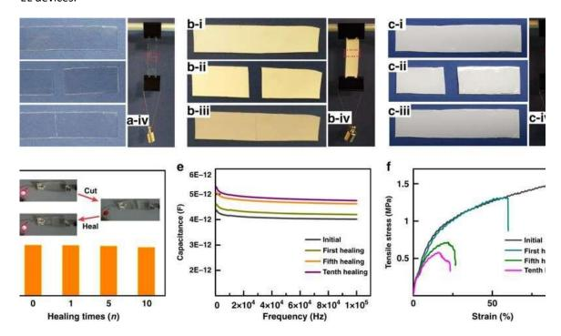
Characterizing the EL device. a—c) Images of the self-healing processes of the EL component layers and the device (PAA layer—a, PU composite layer—b, and EL device—c). In these processes, i) shows the initial states, ii) shows the cut ...more
