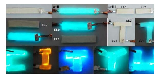
LEGO assembly process of self-healing EL devices. a) A complete EL device was cut into two individual EL units. a-i) indicates the initial resting state, a-ii) the working state, and a-iii) the cut state. b) The as-obtained two EL units in ...more
