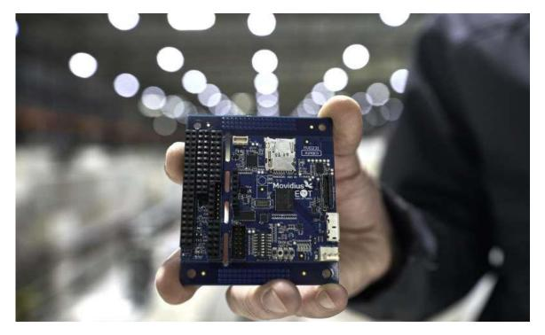
Myriad 2. Credit: CERN/Maximilien Brice"The Myriad 2 requires less than a watt of power, and would also let instruments identify features of interest autonomously – for instance, spotting sudden flood events or forest fires, then realising these need to be sent down to the ground."
