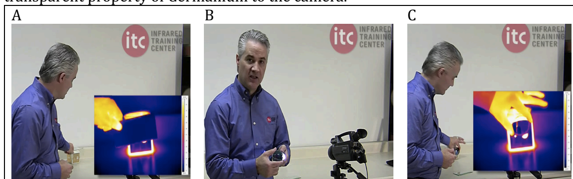
Figure 14. Non-Thermoelectric Germanium. (A) 'Opaque' thermoelectric glass in front of the heat source; (B) visibly opaque germanium in hand; (C) 'transparent' non-thermoelectric germanium placed in front of the heat source [41].
