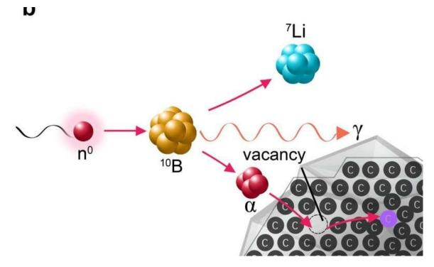
Neutron capture by boron nuclei produces a dense shower of helium and lithium ions, which have the same effect within the nanocrystals as the ions produced in an accelerator: the controlled creation of crystal defects. Credit: IOCB Prague
