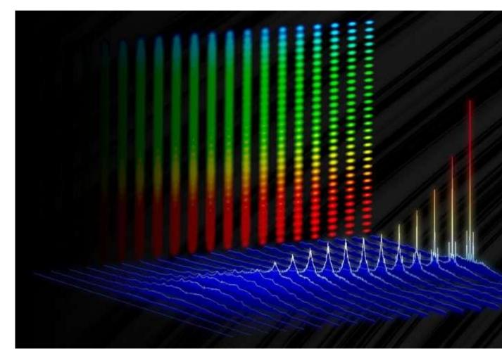
Graphic depicting how specific frequencies, or colors, of light (sharp peaks) emerge from the electronic background noise (blue) in NIST's ultrafast electro-optic laser. The vertical backdrop shows how these colors combine to create an ...<u>more</u>
