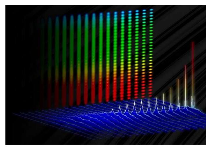
Graphic depicting how specific frequencies, or colors, of light (sharp peaks) emerge from the electronic background noise (blue) in NIST's ultrafast electro-optic laser. The vertical backdrop shows how these colors combine to create an ...more
