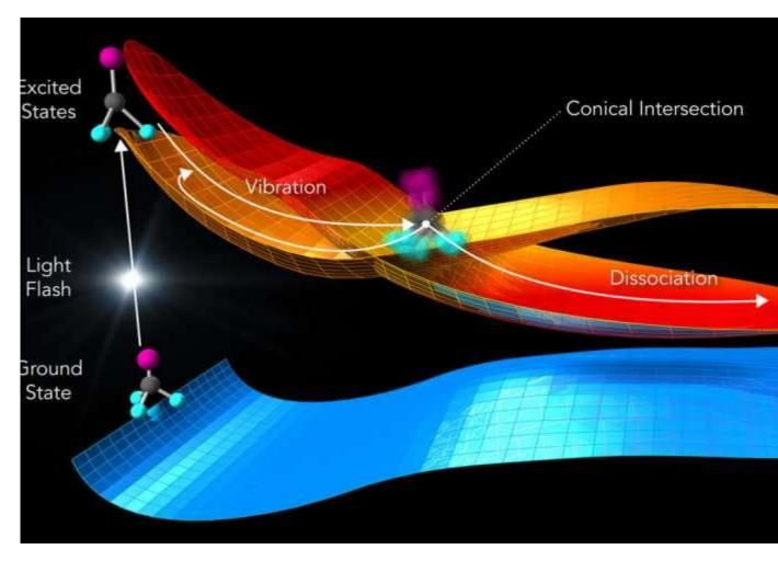
Illustration of the laser-driven response of trifluoroiodomethane molecules (balls and sticks). A laser flash elevates the molecule from a low-energy ground state to an excited state of higher energy (at left). The molecular states are ...more
