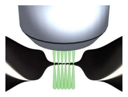
Atoms are shaped into a wire using laser light. Their flow can be influenced by projecting a variable number of light obstacles focussed on the wire with a microscope objective. Credit: Esslinger group/ETH Zurich
