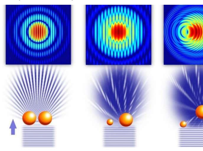
Illustration showing the principle of in-flight holography. (Left) The X-rays scatter off two spheres and form a characteristic diffraction pattern. The patterns are recorded using the very intense X-ray beam of SLAC's X-ray laser, the ...more
