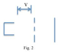
This configuration is essentially the same as the ordinary double slit apparatus with an extended source. We expect to have an interference pattern described by the displacement on the detection screen,  $y \approx \frac{nD}{d}\lambda = \frac{nD}{d}\frac{h}{p}$ , where  $p = m\nu$ ,  $\nu$  is the speed after the particle left the electric voltage area. Configuration 3: the electric voltage is applied on the slit wall only (Fig. 3).
