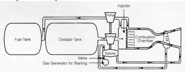
Fig.1. Typical liquid rocket engine.
