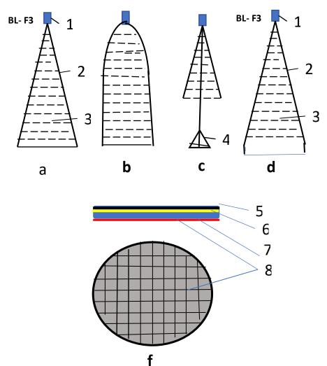
Fig. 3. Suggested Rocket without usual body and engine. *Notations: a, b, c, d* -different versions of the offered rocket, f – fuel layer; 1 – head of rocket, 2 – light cover of fuel, 3 - solid fuel layers, 4 – control of the trajectory direction and rotation; 5 – partition which separated solid fuel layers, 6 - heat insulator, shock absorber, 7 – layer of explosive, 8 - ignition net.
