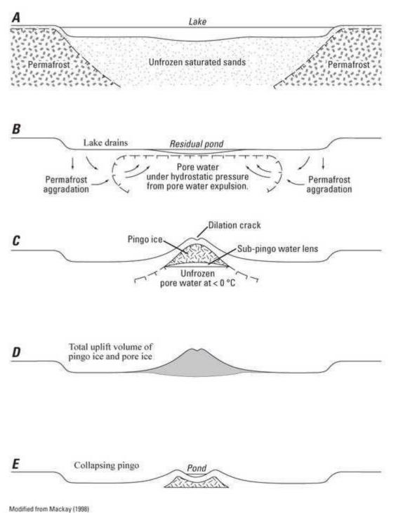
Figure 6. An illustration of collapsing pingos, from the USGS.
