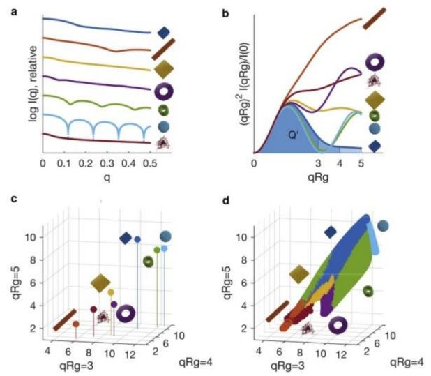
Simulated scattering intensity profiles for different molecular shape classes, shown schematically on the right (a). Reduced form of the intensity profile for each shape class (b). Each shape class defines a point cloud in normalized apparent volume space, with each shape falling into well-defined regions (c, d). (Courtesy: Franke et al Biophys. J. 114 2485 ©2018, with permission from Elsevier)
