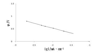
Fig. 2 Cathodic polarization curve of electrolytic process
