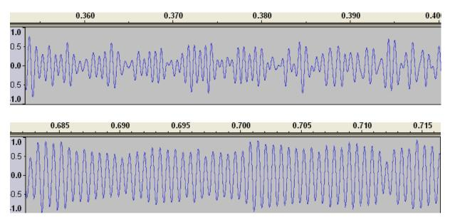
Figure 5. Hold1 above, Hold2 below, synchronized to the same place in everything. Everything on Hold2 is at 0.265-0.615 s and the corresponding place on Hold1 is 0.3-0.65 s.
