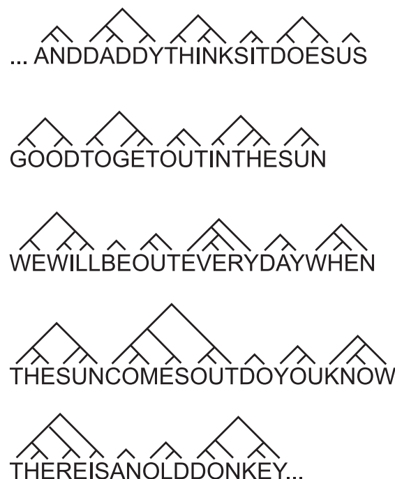
Figure 9: Part of a parsing created by program MK10 [67] from a 10,000 letter sample of English (book 8A of the Ladybird Reading Series) with all spaces and punctuation removed. The program derived this parsing from the sample alone, without any prior dictionary or other knowledge of the structure of English. Reproduced from Figure 7.3 in [70], with permission.
