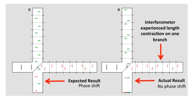
Fig 3.1 – Michelson Interferometer
