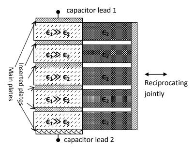
a. cascade mode, total capacitance = embedded\_capacitance/(N+1)
