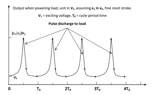
Fig. 2: full loaded voltage output
