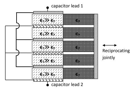
**b.** parallel mode, total capacitance = embedded\_capacitance\*(**N+1**)
