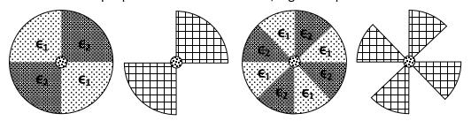
Electrode plates area = **50%** of disc area for many applications
