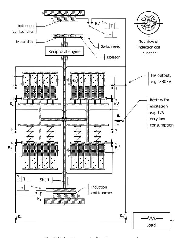
Fig. 8: high voltage periodic pulse power supply
