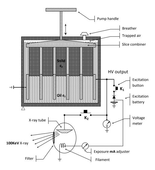
Fig. 10: simple hand pumped hydraulic mobile pulse X-ray source
