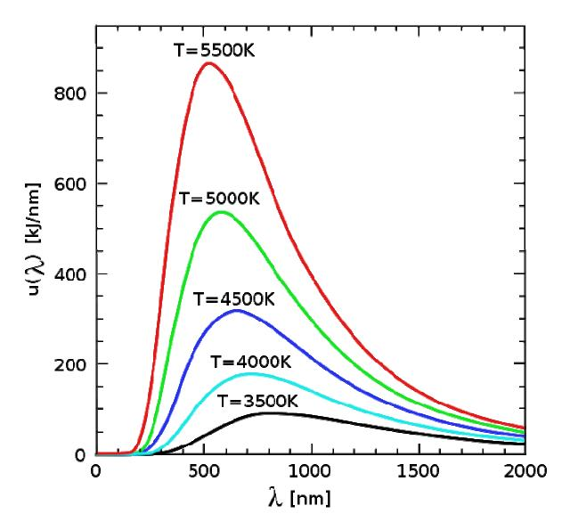
Figure 2. The distribution law for different T temperatures
