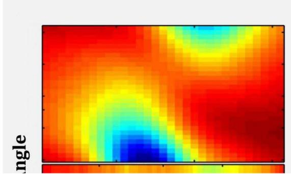
The "plot for experts": the recorded detector image shows that the incident X-ray radiation is amplified particularly at certain angles (blue and green areas). The energy difference between the two resonances that occur is a tiny 37.3 nano-electronvolts.
