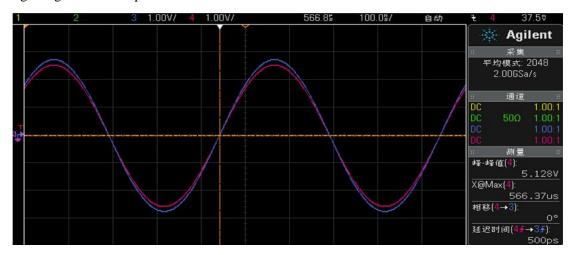
Figure 2, Display of time delay, 6.4 m versus 0.4 m, at 2.0 MHz
