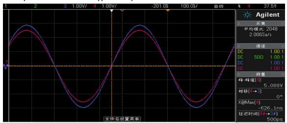
Figure 3, Display of time delay, 9.4 m versus 0.4 m, at 2.0 MHz In Figure 3, the time delay is 0.5 ns.
